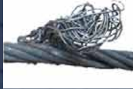
Replace Frayed Cables
